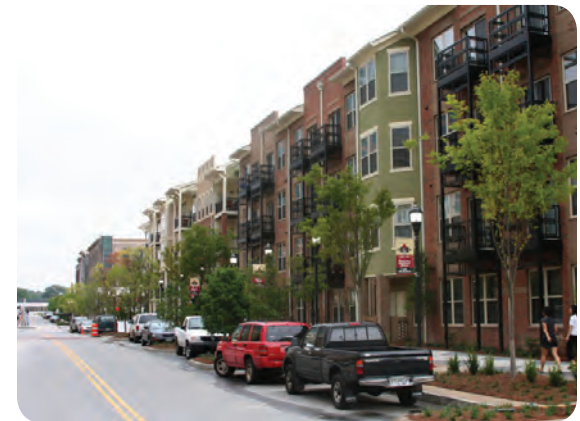
Residential sidewalks are protected from street traffic by planting buffers and on-street parking.
