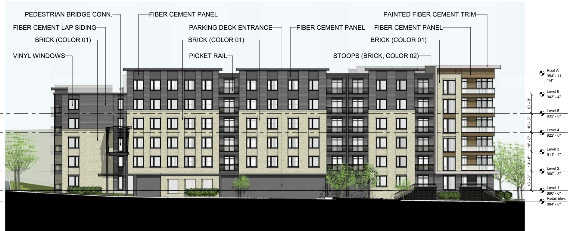
ELEVATION 6 - BUILDING B
