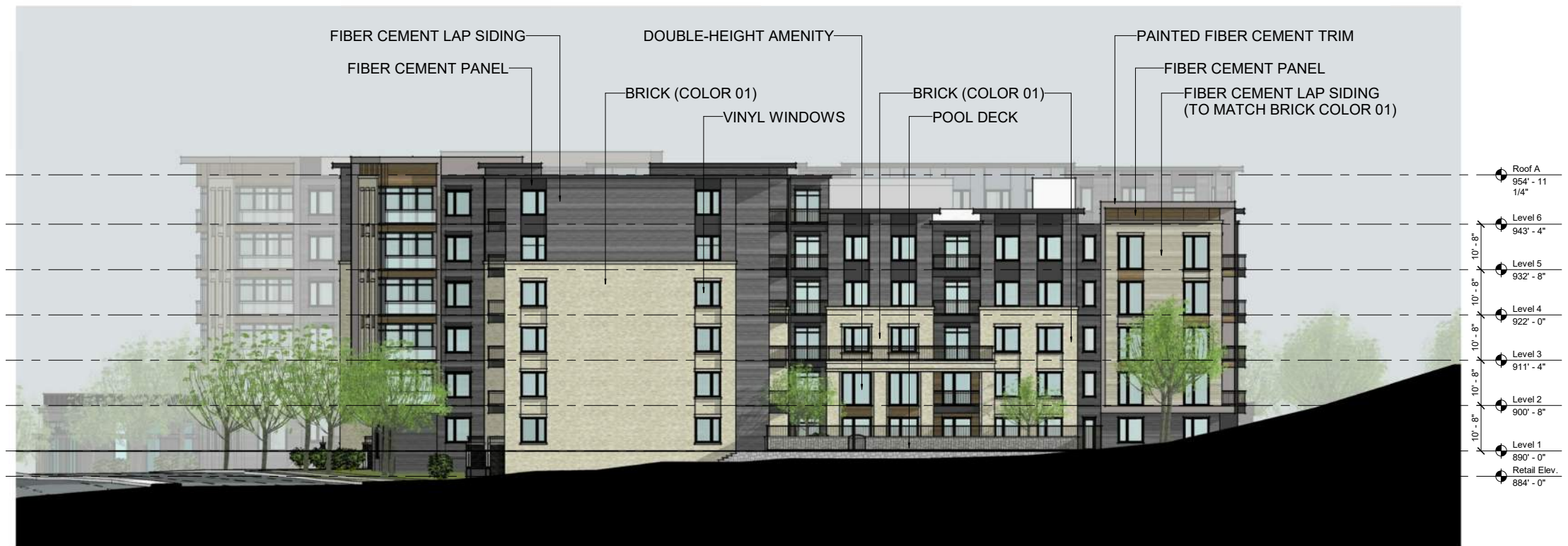
ELEVATION 9 - BUILDING B
