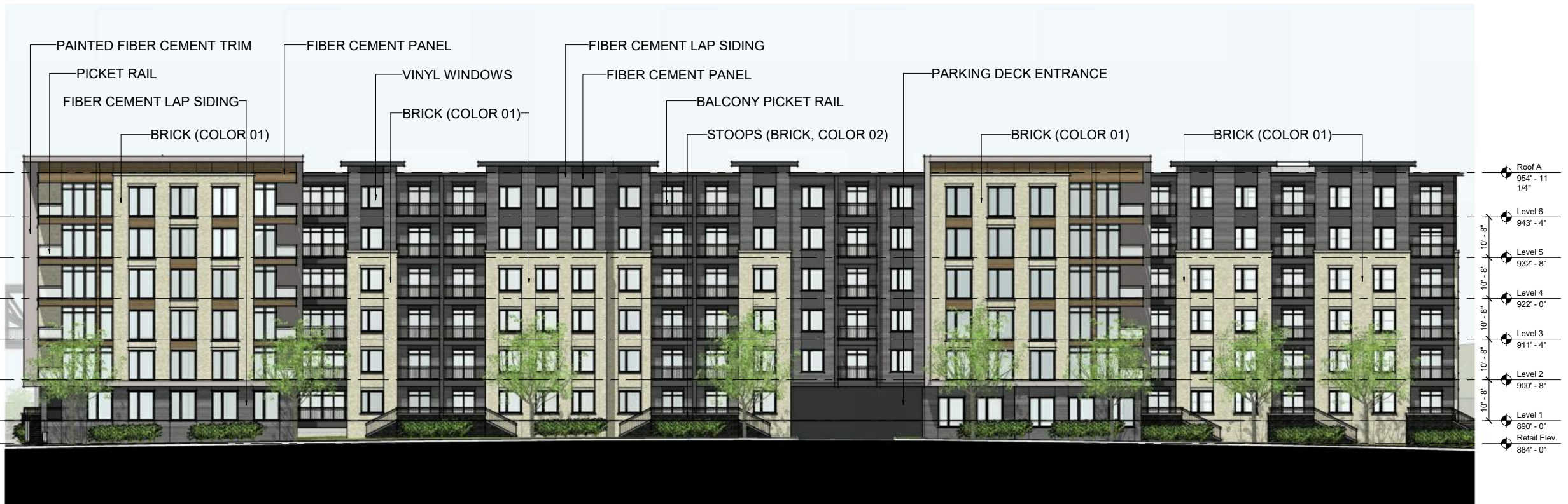
ELEVATION 7 - BUILDING B (CLAIRMONT RD)
