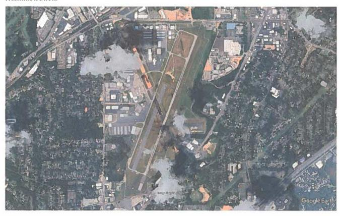
The Airport lies at an elevation of 1,003 feet and contains four active runways and one helipad. Runway 2R/20L is 6,001 feet in length and 100 feet wide with a concrete grooved surface in good condition. Weight bearing capacity is 46,000 pounds single wheel and 75,000 pounds dual wheel. This runway has high intensity runway edge lights, a 4-box VASI on 2R, and a 2-light PAPI, medium
