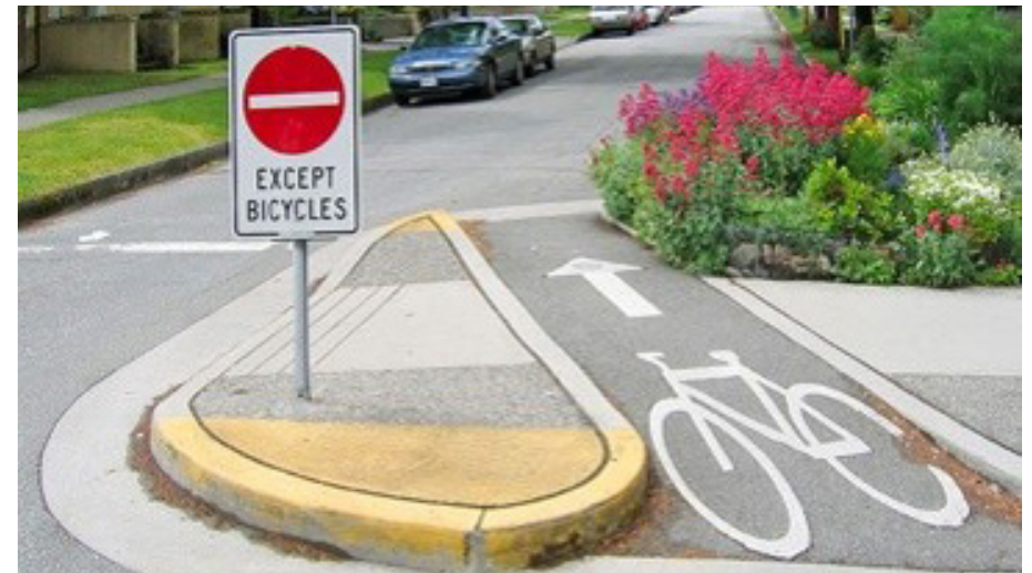
Neighborhood greenway example showing limited vehicle entry while utilizing signage and pavement markings for cyclists.
