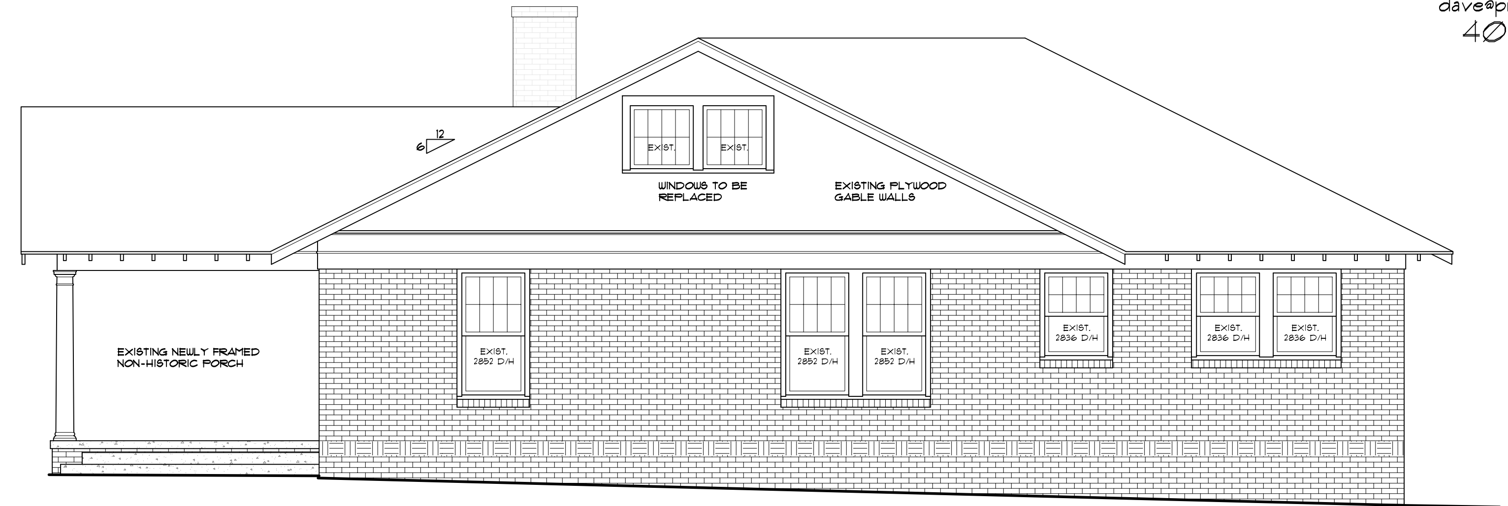
EXISTING NEWLY FRAMED NON-HISTORIC PORCH 12 6 EXIST. 2892 D/H EXIST. 2892 D/H EXIST. 2836 D/H EXIST. 2836 D/H EXIST. 2836 D/H EXIST. 2836 D/H WINDOWS TO BE REPLACED EXISTING PLYWOOD GABLE WALLS WINDOW SHAPE TO BE MODIFIED WINDOWS TO BE REPLACED WINDOW TYPE TO BE MODIFIED WINDOW SHAPE TO BE MODIFIED PRIMARY RIGHT ELEVATION SCALE: 1/4" = 1'-0"
