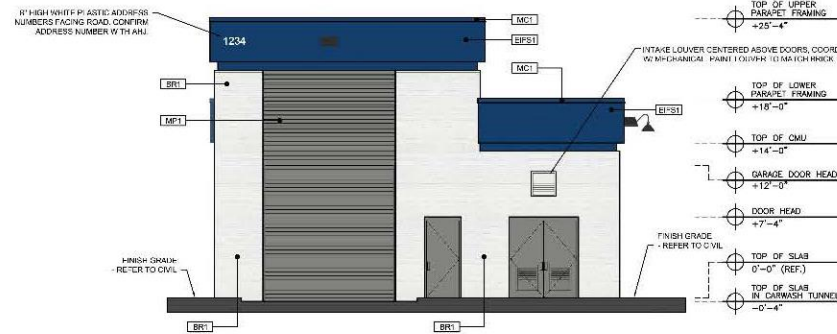
4 EAST (REAR) ELEVATION A2.0 SCALE 3/16" = 1'-0"
