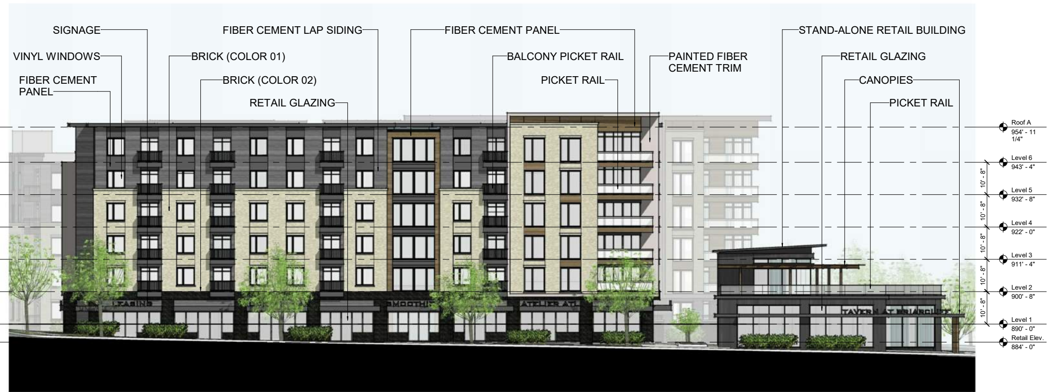
ELEVATION 2 - BUILDING A (BRIARCLIFF RD)
