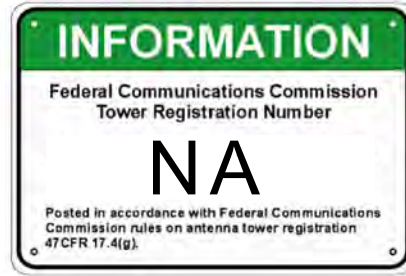
FCC REGISTRATION SIGN WHITE/GREEN BACKGROUND, WHITE/BLACK LETTERING. MOUNTING LOCATION: GATE & BASE OF TOWER. QUANTITY: 2
