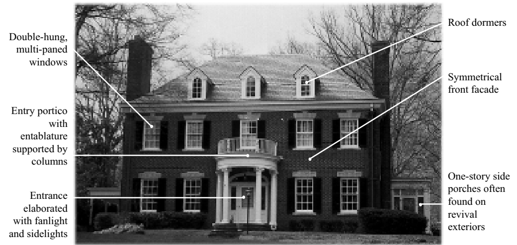
Typical example of the Colonial Revival style with principal features keyed
