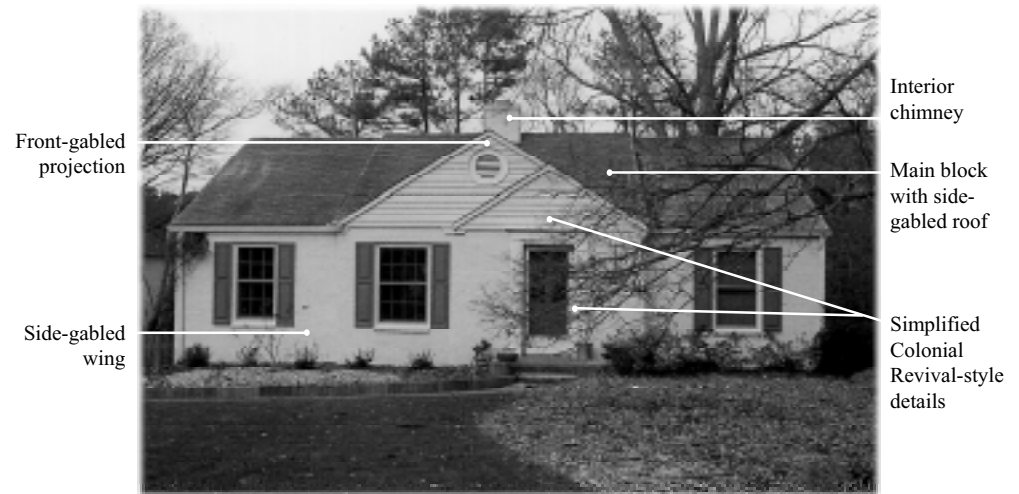
Example of the Emory Grove House Type with principal features keyed.
