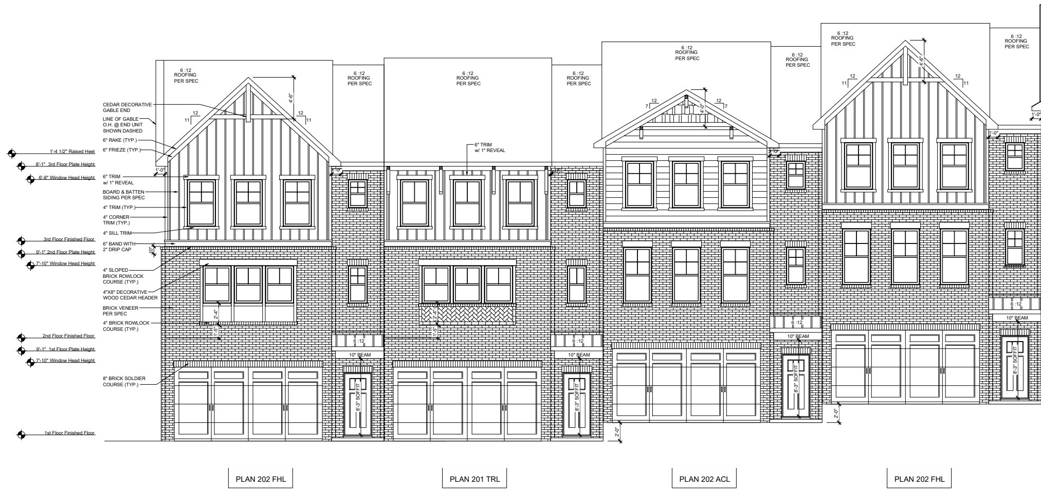
FRONT ELEVATION 7-PLEX SCALE: 1/8"=1'-0" (11"x17" SHEET SIZE) SCALE: 1/4"=1'-0" (24"x36" SHEET SIZE)
