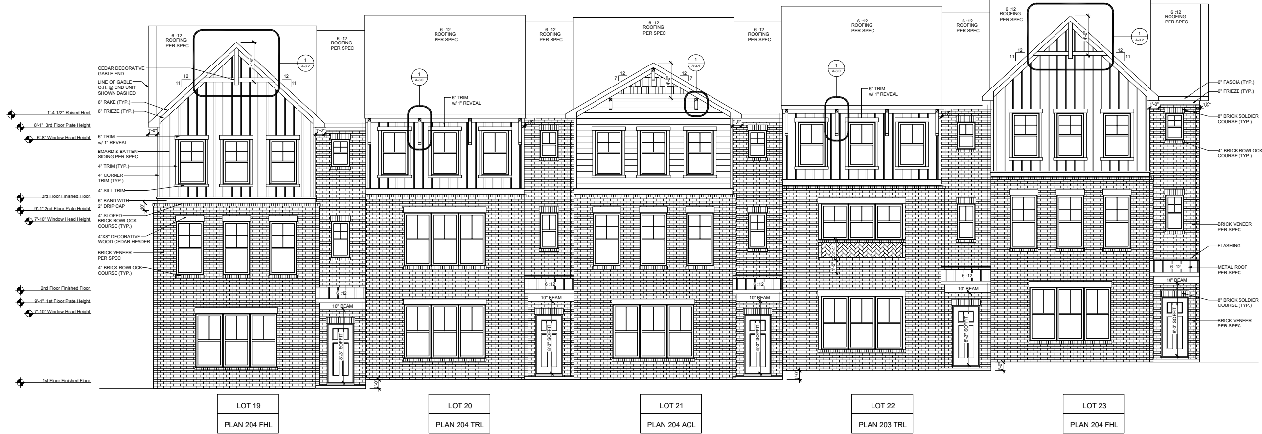
FRONT ELEVATION 5-PLEX LOTS 19-23 SCALE: 1/8"=1'-0" (11"x17" SHEET SIZE) SCALE: 1/4"=1'-0" (24"x36" SHEET SIZE)
