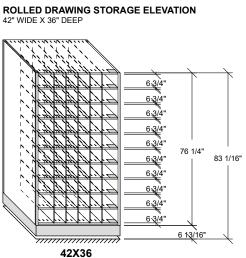
(60) 6X6 OPENINGS PER 42"W UNIT FACE (40) 6X6 OPENINGS PER 30"W UNIT FACE (1,120) OPENINGS TOTAL
