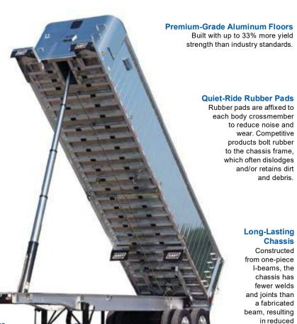
\*\*21-inch aluminum frame is constructed from two T-section beams welded at the center.
