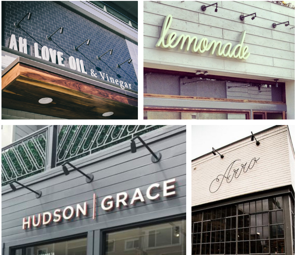
OPTION 4A: Individual Dimensional Letter Forms with Gooseneck External Illumination
